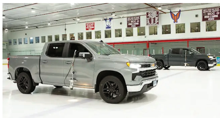
We perform braking tests at a local skating rink to ensure consistent conditions for evaluating ice traction.
