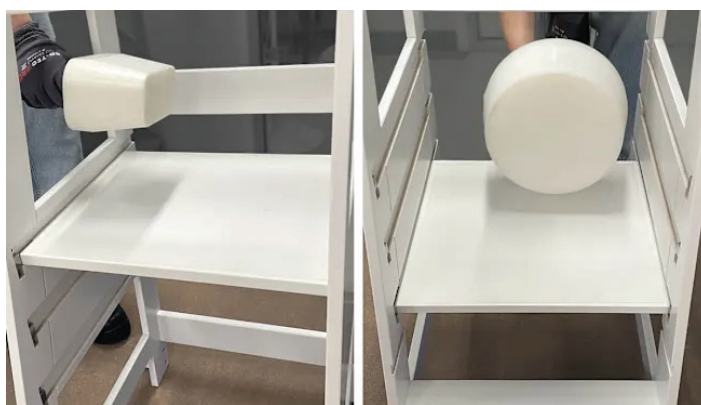
CR's tests used tools the size of a toddler's head (left) and torso (right) to evaluate whether the towers posed an entrapment risk. If a gap was big enough to allow the child's torso to fit through but not their head, that indicated an entrapment risk. Photos: Consumer Reports
